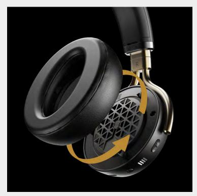
Attach the new earpad and twist clockwise to secure it.
